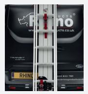
2 belts top and bottom to hold ladder tightly in place and eliminate rattling
