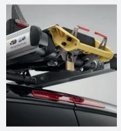
Rubber inserts on the brace bar, reducing rattling noise while in transit \*A padlock can be added\*
