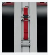
Beltstow system to secure strap when not transporting a ladder
